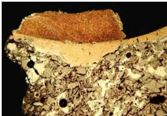
Figure 8: Section through a scorifier, with a droplet of lead left over on the surface. The bright layer underneath is lead oxide formed during the scorification process, which appears badly penetrating through the sand-tempered ceramic. The lead particle shows dendrites of silver (brightest phases) precipitated from the lead upon cooling, showing that the concentration of the precious metal took place in spite of the relatively poor quality of the ceramic plate. The width of the lead particle is about 1 mm. Photomicrograph under reflected light, 50x magnification.
